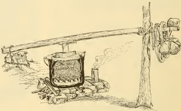
FIG. 6.—Use of the lever in pressing wax.
